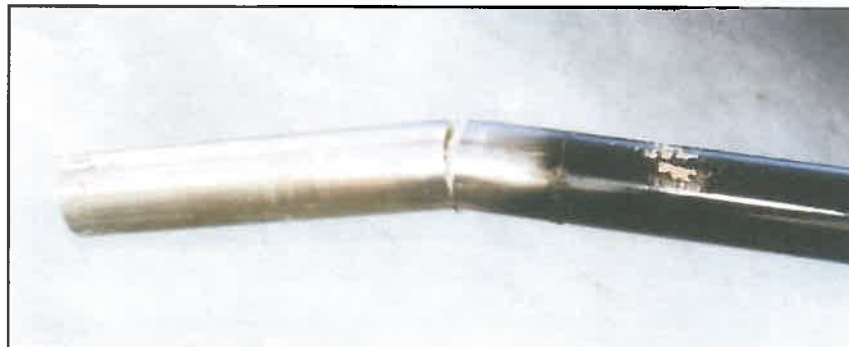
Photo 6d. Post-test Close-up Of The Exemplar Pole Containing The Reinforcing Bar In The Concrete.
