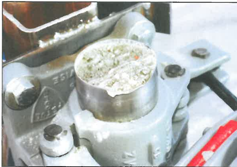
Photo 6c. Close-up Of Failure Of Machined Exemplar Pole
