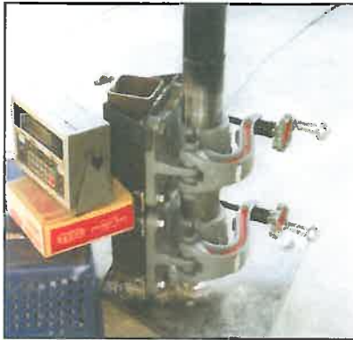
Photo 6a. Machined Exemplar Pole In Clamp, Prior To Test.
